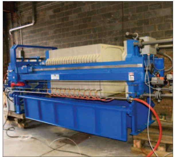
Figure 2: A typical filter press
